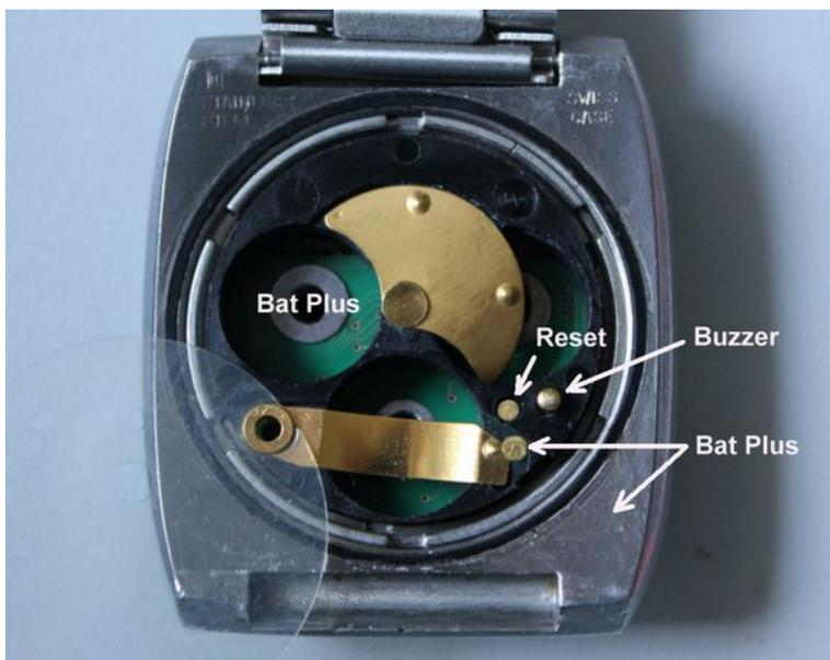
Battery Plus must be connected to the case, the contact is established by the inner ring. The Buzzer and Reset may not be connected to Bat Plus. Check that there is no contact between them. If there is any contact, you have to turn the battery case until it is exactly horizontally and you have to check the correct location of the spring contacts, which of course cannot be seen below the battery holder.
