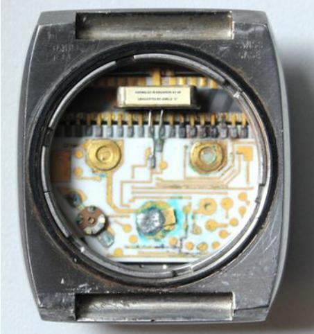
Next you have to remove the outer ring. This ring has a left handed thread. You have to move it **clockwise!** Again use tweezers or your special needle-pliers to make the first turn. After some turns you have to loosen the front housing against the back housing and go on, before the two housings can be separated. Remove the outer ring, which is split at one side.
