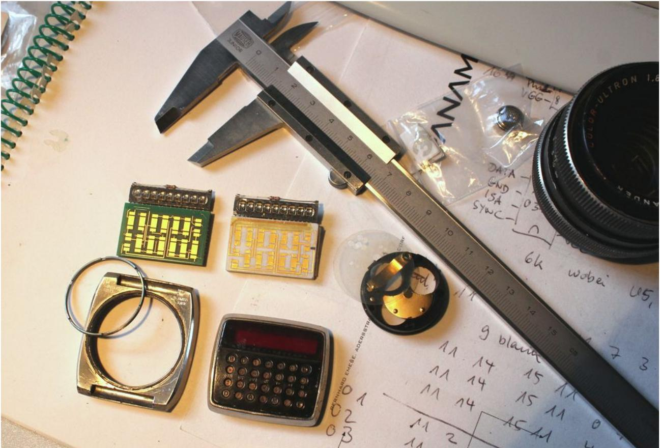
Your repair kit consists of the processor board and the keyboard. They are already attached together and connected by 11 copper wires, but not folded, because this can be done only after the display is mounted. The Real Time Clock chip PCF2127 was filed off on both sides by about 1 mm before assembly, otherwise the board would not fit into the watch case later.
