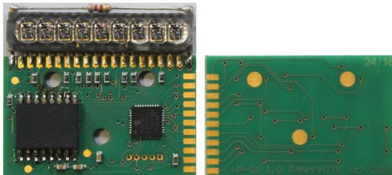
Both have gold plated contacts and need to be put together by 11 wires and be fixed perfectly aligned in 1 mm distance. Because the display has to be soldered to the lower processor board before attaching and fixing the upper board, there is no easy way to Do It Yourself. But anyway it is described here how to do it the best way.
